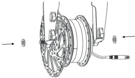
4. Fasten clockwise BC3/8 cap lock-nuts with open-end wrench at both ends of the motor. Torque requirement: 30-36N.m.
