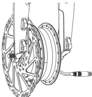
3. Mount one 2mm washer on both sides of the frame.
